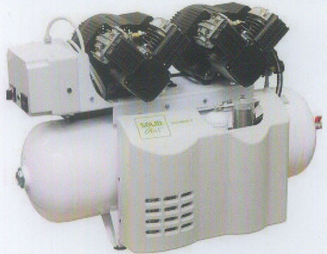
Model 500AT-T, 2x2.4hp, 2x1.8kW, 2x188L/min, 13.2cfm, 68dB(A) on 100ltr tank
