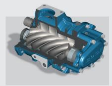
With its innovative profile geometry (5:6 screw profile), the BOGE effilence maintains a low differential pressure between the chambers and thus achieves excellent volumetric efficiency.
