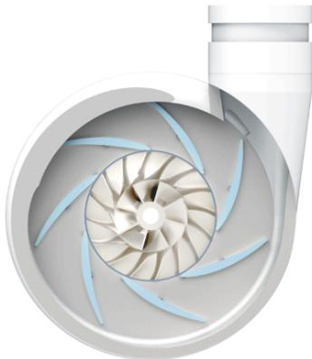
Unlike magnetic bearings or roller bearings, a shaft with air-lubricated bearings does not need either external power or any material other than air to achieve extremely high speeds. The air-lubricated bearing stabilises itself and does not require any auxiliary bearings. In addition, this type of bearing ensures virtually wear-free operation and a correspondingly low amount of maintenance.
